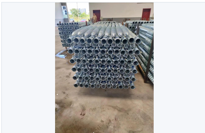
Hot-dip galvanized and packaged ground screws – final inspection before shipment.
