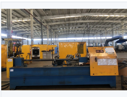
Semi-automatic steel strip welding machine – welding of threaded steel strips.
